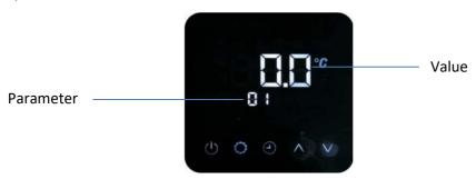
Use the UP  $\wedge$  button to scroll through the parameters. The parameters available to view are as shown below with their corresponding parameter numbers.
