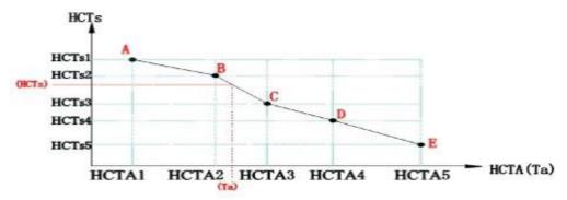
be above HCTA1, and below HCTA3. If a mistake is made when entering the values, and this is not followed, the value will automatically be corrected by the controller.
