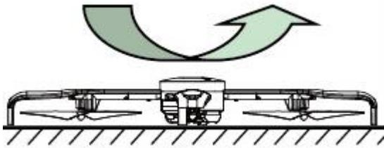
2. With the drone level, rotate it anticlockwise for 3 full revolutions. The lights at the rear of the drone will illuminate.
