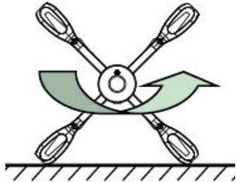
For accuracy the GPS should be calibrated before each flight, and we would advise that the drone is at least 50cm away from the ground during calibration.
