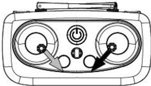
To do this push the left joystick to the bottom right position at the same time as pushing the right joystick to the bottom left position.
