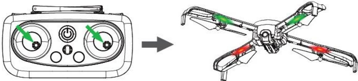
Release the joystick, which will complete the calibration.
