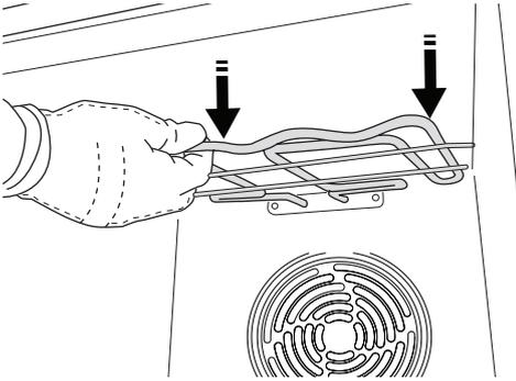
To return the heating element to its position, lift it up, pull it slightly towards you and make sure that the tab support is in its proper seating.
