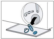
**3.** Ensure that both impellers can turn.
