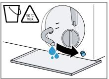
8. Firmly press on the sealing cap.
