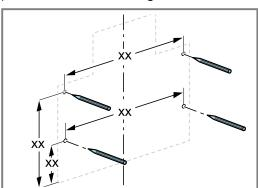
The bottom edge of the appliance is identical to the lower edge of the drilling template.
