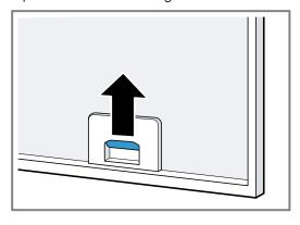
Remove the grease filters from the holders.
