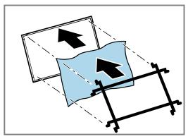
Use the grid to secure the odour filter to the outer holes.
