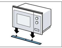
**3.** Screw the middle screw tightly on the base of the microwave.
