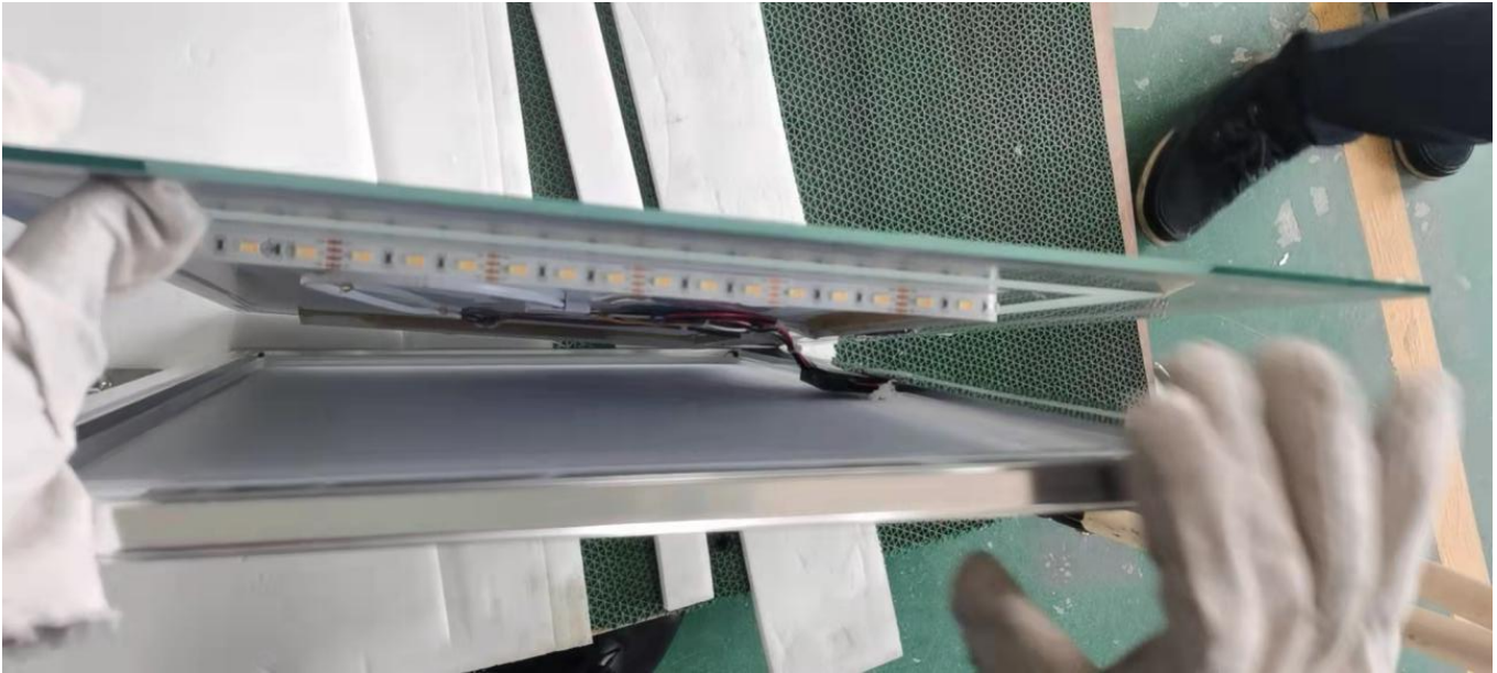
4. Cut all the 4 adhesive edges, and separate the mirror from the aluminum frame
