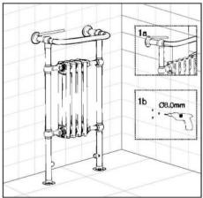
**Please note:** If drilling into tile, it is recommended to tape the wall to prevent the drill from slipping.
