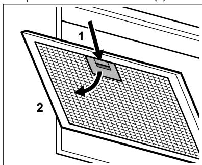
2. Slightly tilt the front of the filter downwards (2), then pull.
